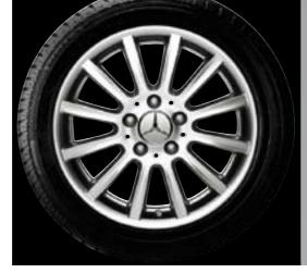
On all light-alloy wheels, use wheel bolt A211 401 0370 and the corresponding rim lock B6 647 0155.
